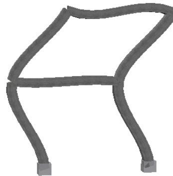
Figure 5-9 B showing the 2nd mode shape frame 3 in Seismostruct
