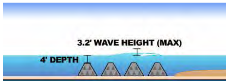
Figure 28: Illustrations showing how wave attenuation devices reduce wave height and impact on shoreline
