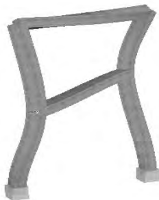
Figure 5-9 C showing the 3rd mode shape frame 3 in Seismostruct
