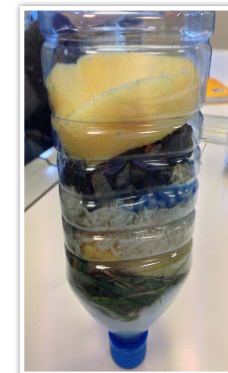
Illustration 23: Homemade water filtration system
