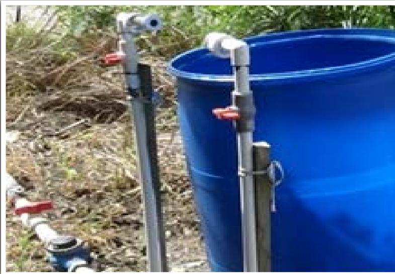
Photo 1: Irrigation head showing meter (on ground) and open space for fertilizer injector
