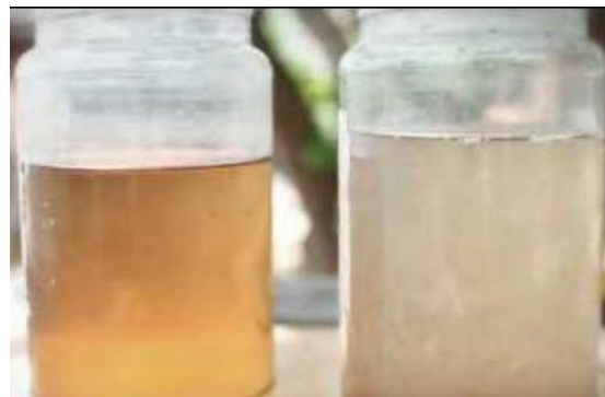
Photo 34: Crushed moringa seeds will clarify murky water
