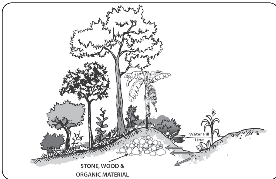
Illustration 2: Demonstrates the position of the berm on the contour bund. This is the most common form of hillslope cultivation in the region.
