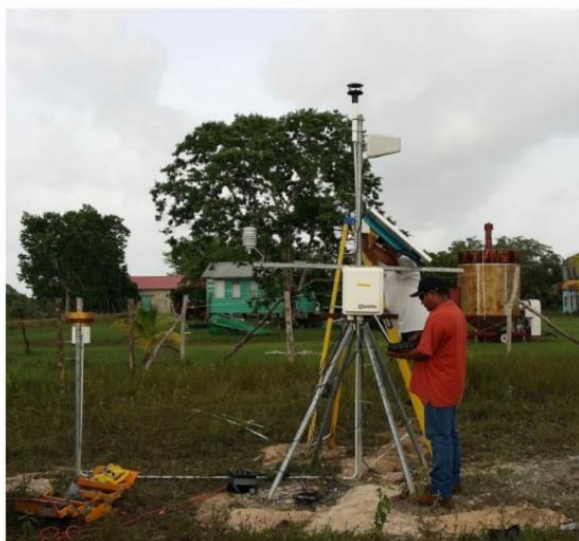
Installation of the first automatic weather station for testing
