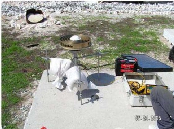
Global Positioning System (GPS) measuring aseismic strain accumulation at Pedro Cay
