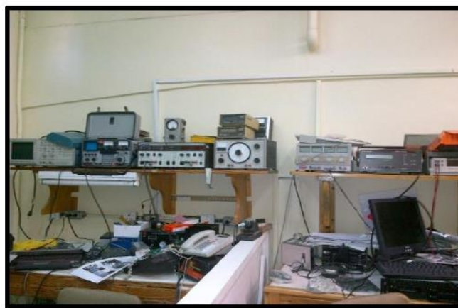
Plates 9 & 10: Loose electrical wiring at work stations
