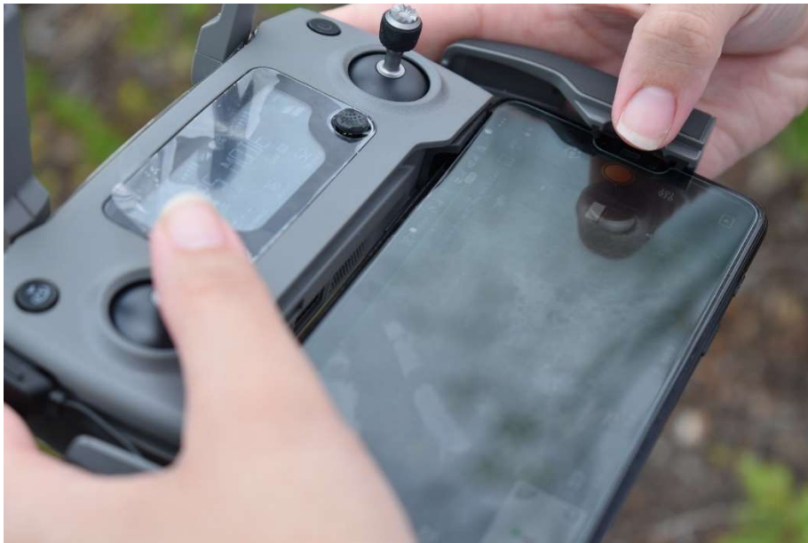
Figure 3: A photograph of the control scheme of a low-cost drone (DJI Mavic 2 Pro, smartphone & controller setup) where aerial footage of an island in The Bahamas was collected to assess damage to the environment. Image credit: The Bahamas National Trust, 2020.
