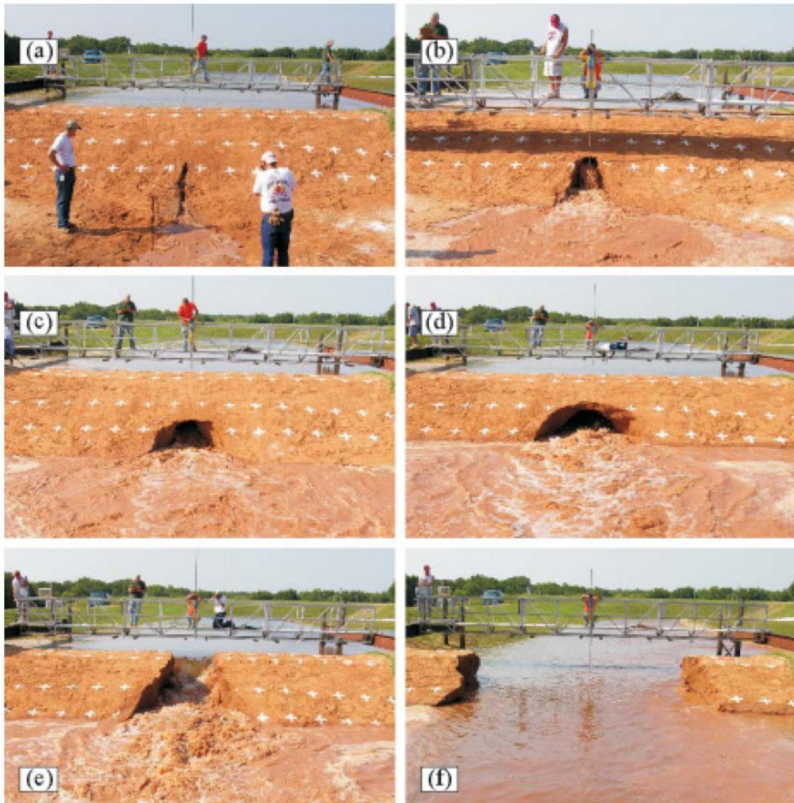
Figure 2-10: Internal erosion failure and breach progression of an embankment dam (West, et al., 2018)
